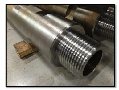
Matrix manufactures dual tube and single tube drill collars in standard and custom configurations. Drill collars add weight to the bit and keep the drill string in tension. This results in straighter boreholes and minimizes dangerous compressive stresses in the drill string.
